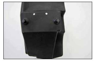
11. Install two airbox mounts onto the  $K\&N^{\otimes}$  airbox with provided hardware.
