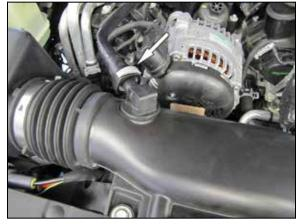
3. Disconnect the crank case vent line.
