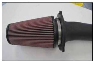
14. Install the K&N<sup>®</sup> air filter onto the K&N<sup>®</sup> intake tube.
