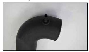
13. Remove the inlet air temp sensor from the factory inlet tube. Then remove the "O" ring from the sensor. Install the provided grommet onto the K&N® intake tube. Then install the inlet air temp sensor into the grommet.
